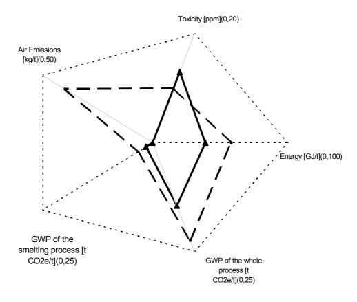
Fig. 1. Comparison of economical and environmental factors in aluminium production by Hall-Herault process (---), and ILs utilizing process (----)
